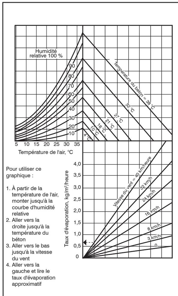
Figure 2.1.5, ACI 305, Hot Weather Concreting
